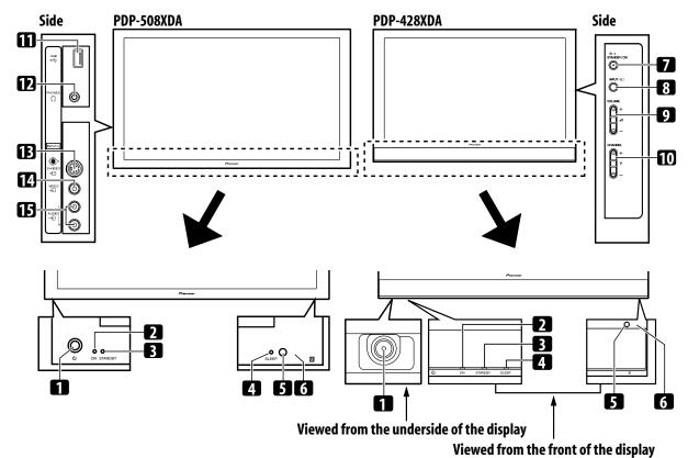
The terminals on side panels are common to the PDP-508XDA and PDP-428XDA.
